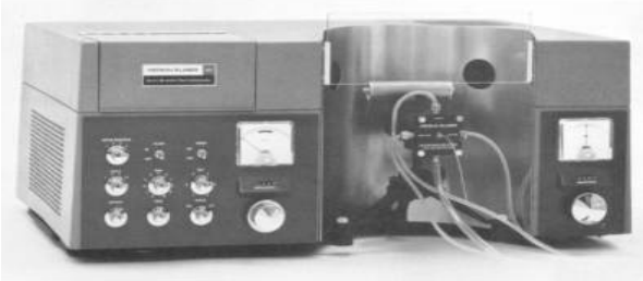
First AA was PE 303 purchased in 1964. It was one of the instruments I trained on.
